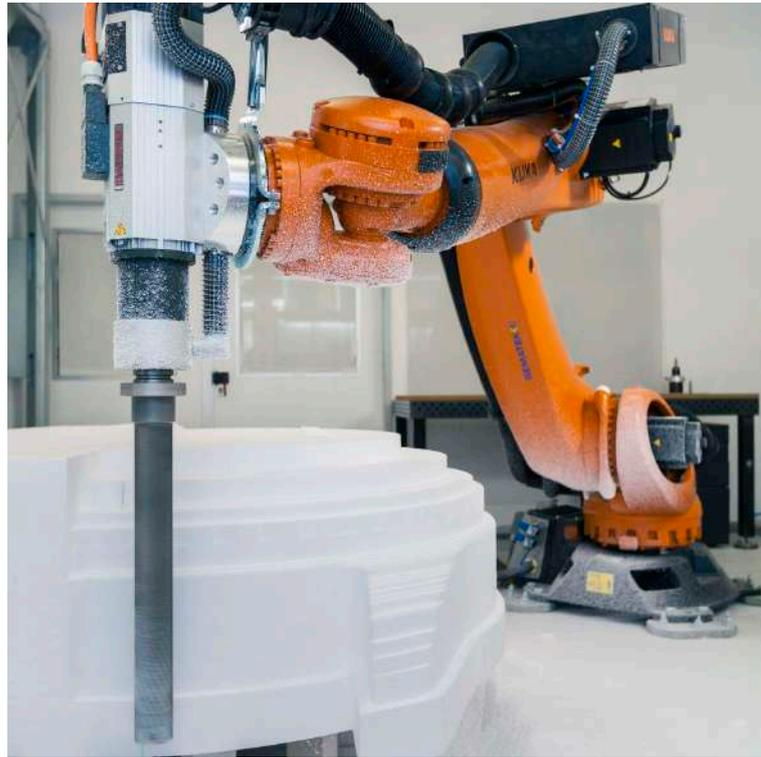
**Fig. 12-1: Robot milling**
