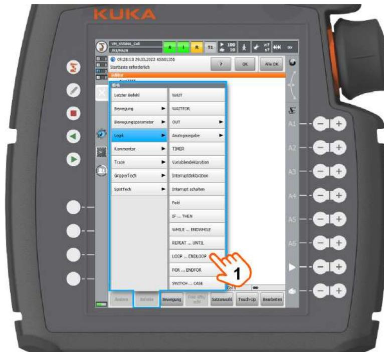
**Fig. 22-3: Programar LOOP-ENDLOOP, paso 3**
