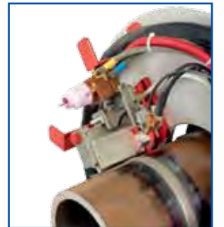
Quick change of the electrode
